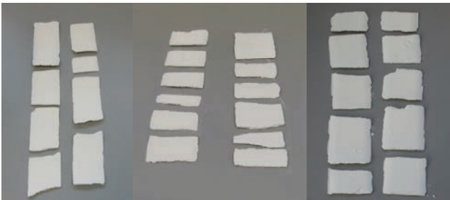
MCC 101 PROSOLV® SMCC 50 PROSOLV® SMCC 50 LD Observation: MCC 101, PROSOLV® SMCC 50 and PROSOLV® SMCC 50 LD yield nicely shaped hard compacts at 25kN compaction force. From above picture we can conclude that PROSOLV® SMCC 50 LD yields dense compacts compare to Microcrystalline cellulose.
