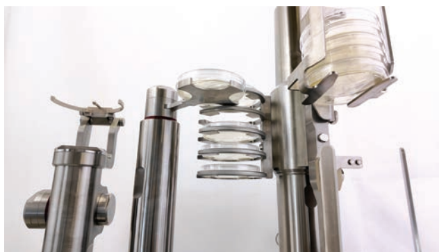
Automated handling transfers each Petri dish from the internal buffer to the monitoring position, where it is opened, scanned and documented. After the defined exposure period, the dish is automatically closed and moved to a separate storage position
