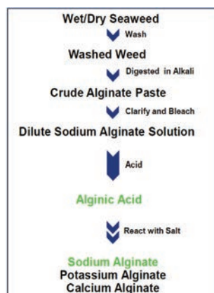
Image 1: Manufacturing process of VIVAPHARM® Alginates [4]
