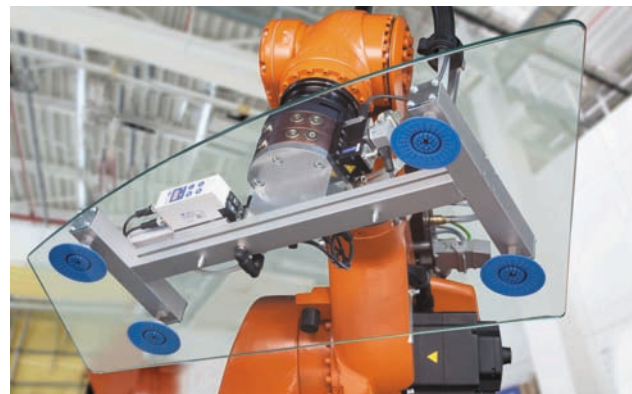
Air Saving Solution at Glass Gluing station
