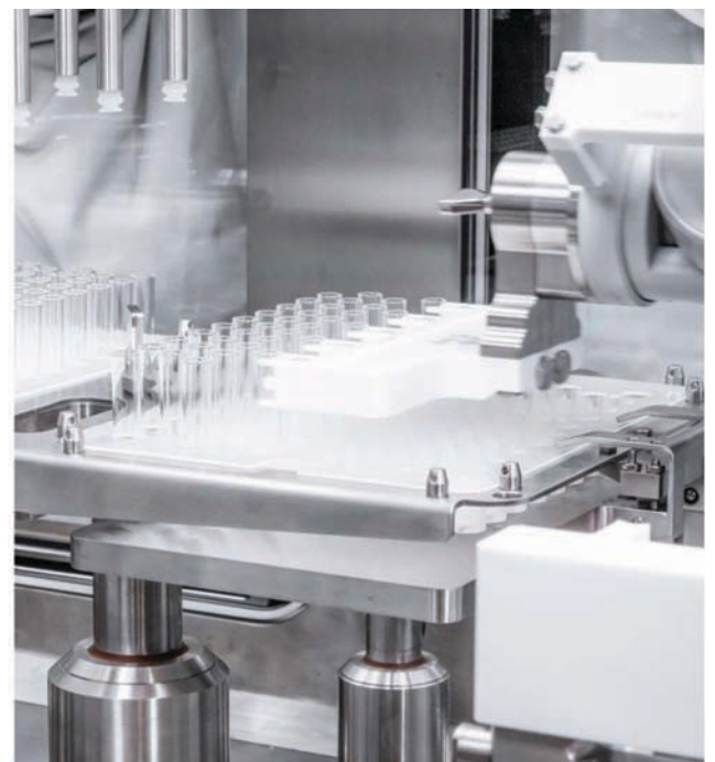
Transfer of the containers into the highly flexible transport system. There is no glass-to-glass contact at any time in the MultiUse lines
