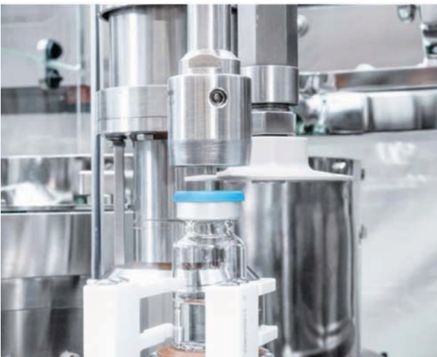
Freeze-dried or liquid? MultiUse: Both product paths can be processed at a common crimping station for vials
