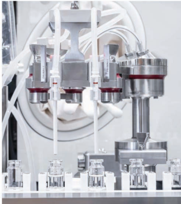
Highly precise dosing system, exact filling volume: If a fill volume is inaccurate, the container is immediately refilled instead of rejected – the so-called “re-dosing on request”
