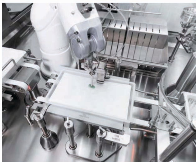
Nested containers are unpacked automatically. Bulk containers such as non-pre-sterilized vials can optionally be fed via a second product path
