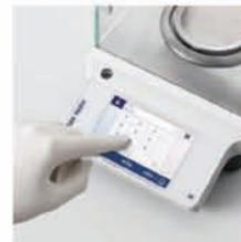
**Intuitive Touch -Operation-**Sample IDs and passcode protection make sure settings are not changed by unauthorized personnel.
