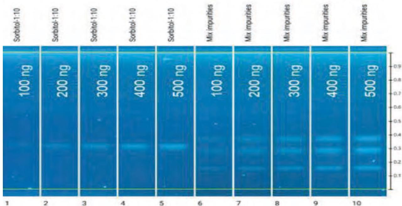
Image at 366nm after derivatization-Sorbitol on tracks 1-5, maltitol, Iditol and mannitol on tracks 6-10, with increasing RF values (Plate applied and developed in CAMAG HPTLC PRO)
