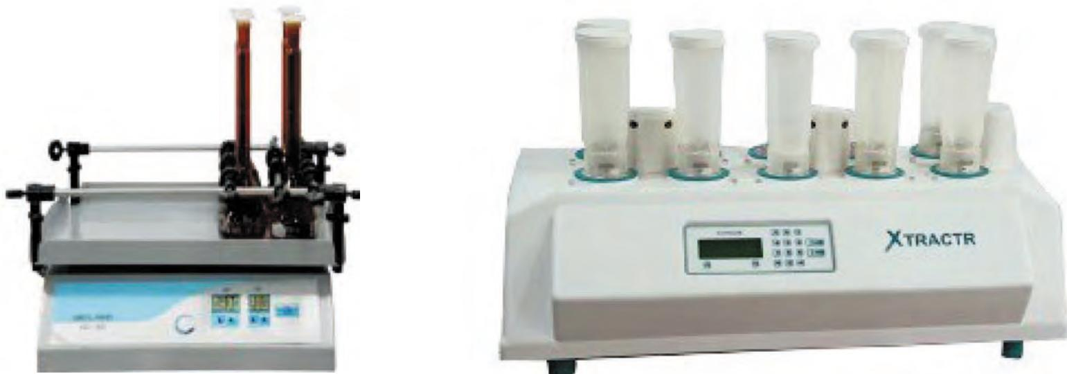
Figure 1: Setup for manual extraction (left) and Xtractr (right)
