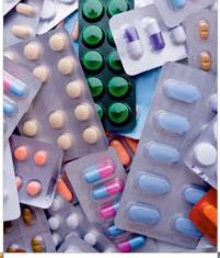
PVC/PE/PVdC **Triplex Laminate Very Good Barrier**
